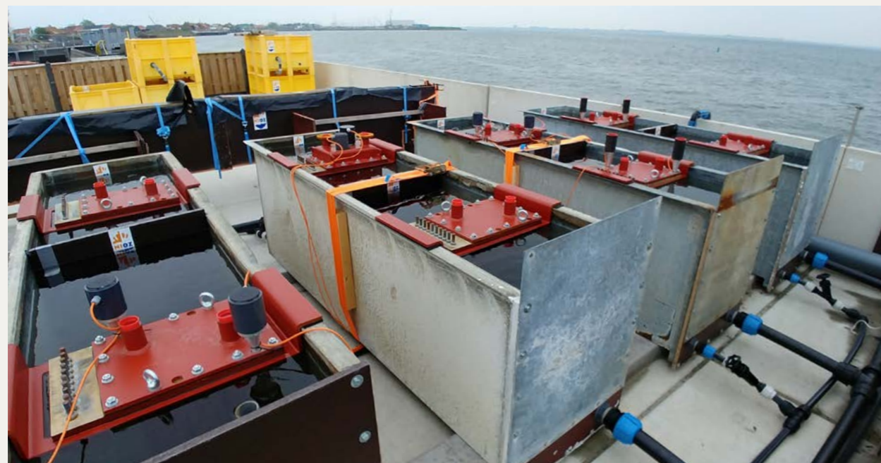
Research setup box-cooler protection
